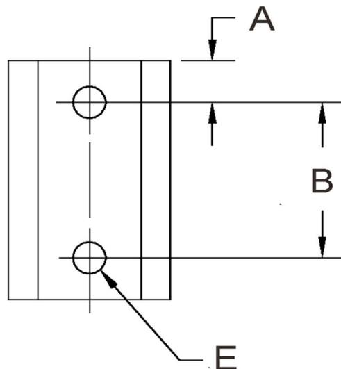
ALL DIMENSIONS ARE TO BE MEASURED WITH THE SPRING CLIP SECURED TO A FLAT SURFACE AND A COMPONENT OF THE NOMINAL DIAMETER IN PLACE.
