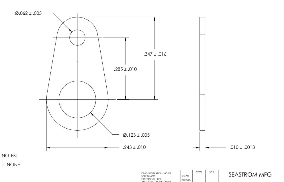
ANGULAR: MACH±1/2 Deg TWO PLACE DECIMAL ±.01 ENG APPR. **RETAINING WASHER** THREE PLACE DECIMAL ±.005 PROPRIETARY AND CONFIDENTIAL MFG APPR. THE INFORMATION CONTAINED IN THIS MATERIAL Q.A. DRAWING IS THE SOLE PROPERTY OF **BRASS** COMMENTS: SEASTROM MANUFACTURING. ANY REPRODUCTION IN PART OR AS A WHOLE SEE NOTE 1 SIZE DWG. NO. 5758-31 WITHOUT THE WRITTEN PERMISSION OF SEASTROM MANUFACTURING IS PROHIBITED. DRAWING IS NOT TO SCALE
