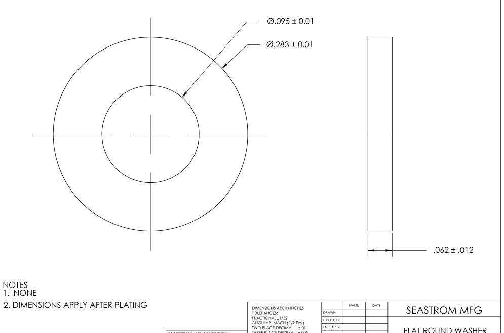
TWO PLACE DECIMAL ±.01 THREE PLACE DECIMAL ±.005 FLAT ROUND WASHER PROPRIETARY AND CONFIDENTIAL MFG APPR. THE INFORMATION CONTAINED IN THIS MATERIAL Q.A. DRAWING IS THE SOLE PROPERTY OF NEOPRENE COMMENTS: SEASTROM MANUFACTURING. ANY REPRODUCTION IN PART OR AS A WHOLE SIZE DWG. NO. 5613-8-62 WITHOUT THE WRITTEN PERMISSION OF SEE NOTE 1 REV. SEASTROM MANUFACTURING IS PROHIBITED. DRAWING IS NOT TO SCALE SHEET 1 OF 1
