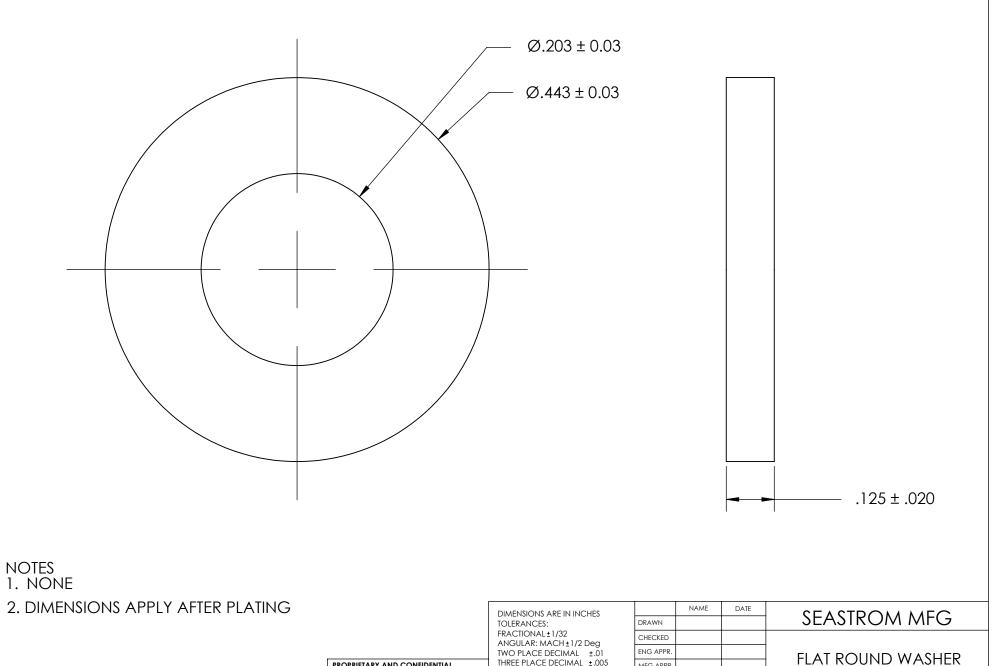
TWO PLACE DECIMAL ±.01 THREE PLACE DECIMAL ±.005 PROPRIETARY AND CONFIDENTIAL MFG APPR. THE INFORMATION CONTAINED IN THIS MATERIAL Q.A. DRAWING IS THE SOLE PROPERTY OF NEOPRENE COMMENTS: SEASTROM MANUFACTURING. ANY REPRODUCTION IN PART OR AS A WHOLE SIZE DWG. NO. 5613-33-125 WITHOUT THE WRITTEN PERMISSION OF SEE NOTE 1 SEASTROM MANUFACTURING IS PROHIBITED. DRAWING IS NOT TO SCALE
