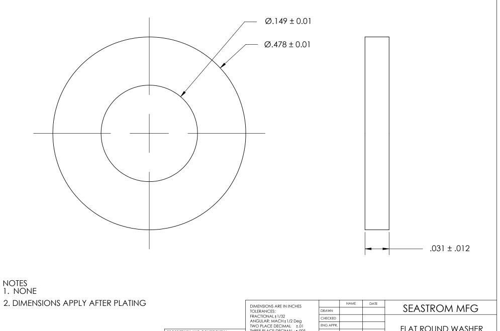
TWO PLACE DECIMAL ±.01 THREE PLACE DECIMAL ±.005 FLAT ROUND WASHER PROPRIETARY AND CONFIDENTIAL MFG APPR. THE INFORMATION CONTAINED IN THIS MATERIAL Q.A. DRAWING IS THE SOLE PROPERTY OF NEOPRENE COMMENTS: SEASTROM MANUFACTURING. ANY REPRODUCTION IN PART OR AS A WHOLE SIZE DWG. NO. 5613-21-31 WITHOUT THE WRITTEN PERMISSION OF SEE NOTE 1 REV. SEASTROM MANUFACTURING IS PROHIBITED. DRAWING IS NOT TO SCALE SHEET 1 OF 1
