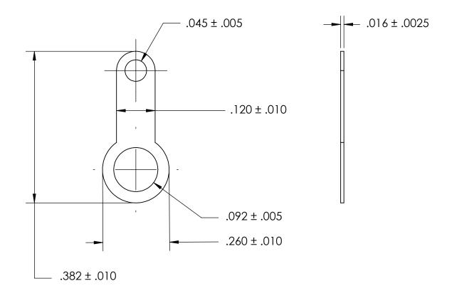
NOTES 1. TIN-LEAD DIP PER MIL-DTL-14072, M258. MUST CERT SOLDERABILITY TO MIL-STD-202, M208 - REFLOW ALLOWED, IF REQUIRED
