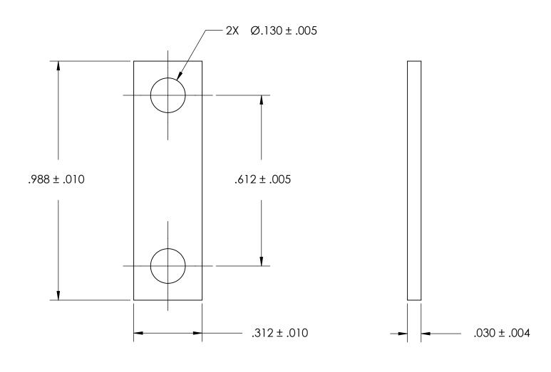
NOTES 1. BLACK OXIDE PER MIL-DTL-13924, CLASS 4, LIGHT OIL, NO TEST REQUIRED
