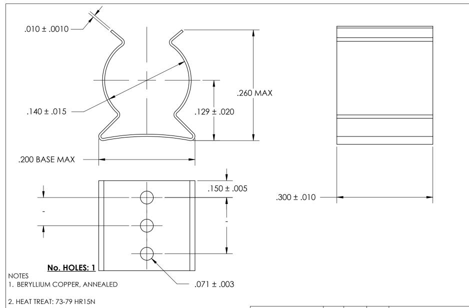
3. SILVER PLATE PER ASTM B700 TYPE 1 GRADE A CLASS S, 2.5µm TH W/NICKEL UNDERPLATE
