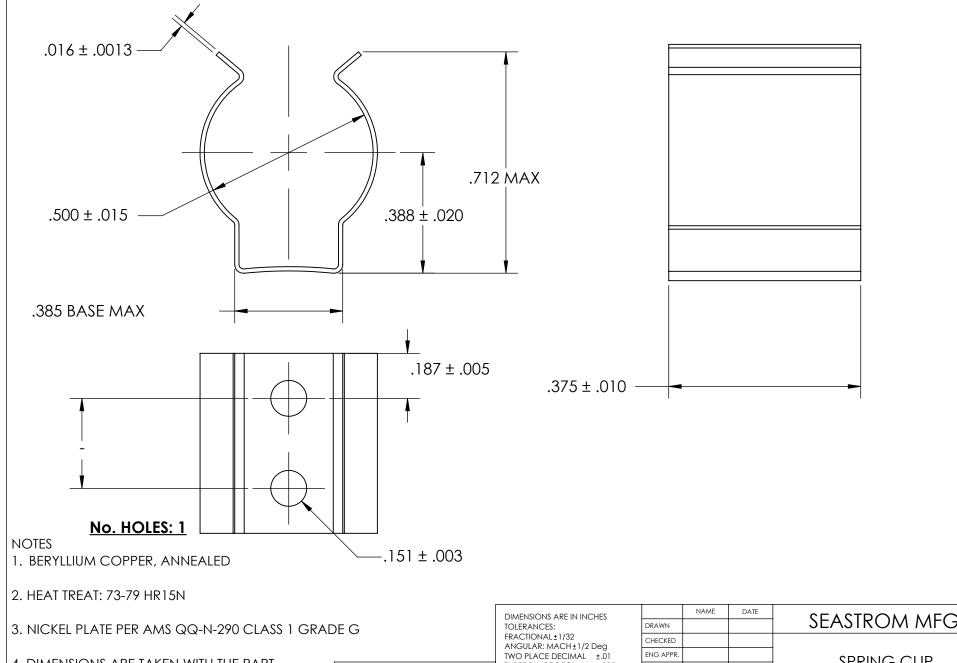
4. DIMENSIONS ARE TAKEN WITH THE PART CLAMPED TO A FLAT SURFACE AND A DUMMY COMPONENT IN PLACE.
