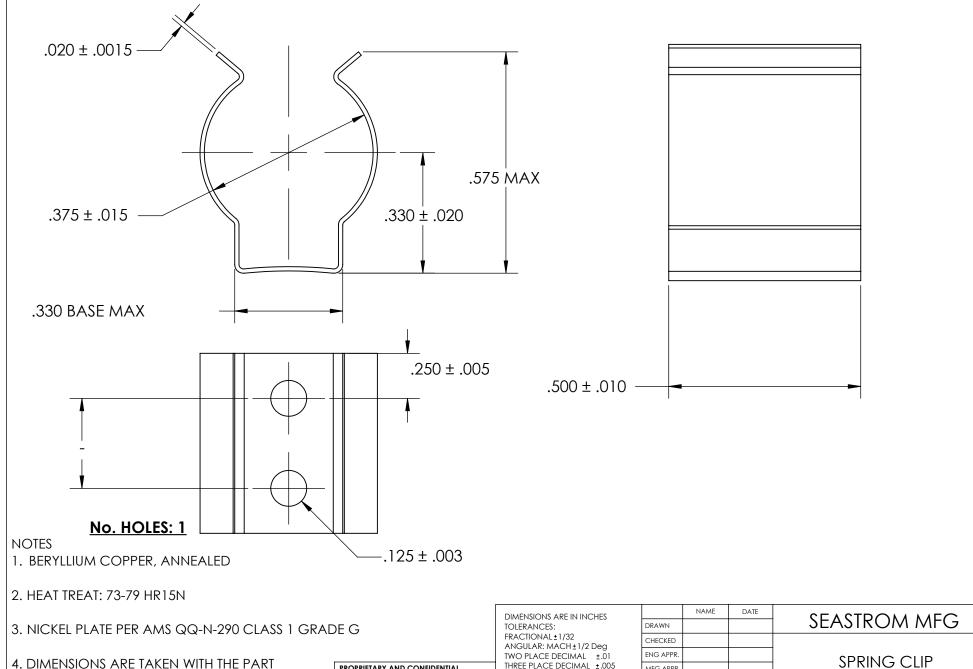
COMPONENT IN PLACE. 5. DIMENSIONS APPLY PRIOR TO PLATING.
